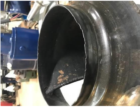
IMPELLER NECK WORN BEYON REPAIR
