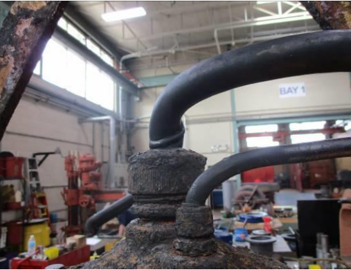
POWER CABLE CUT AND JACKET DRY ROT
