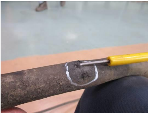
IMPELLER NECK WORN BEYON REPAIR
